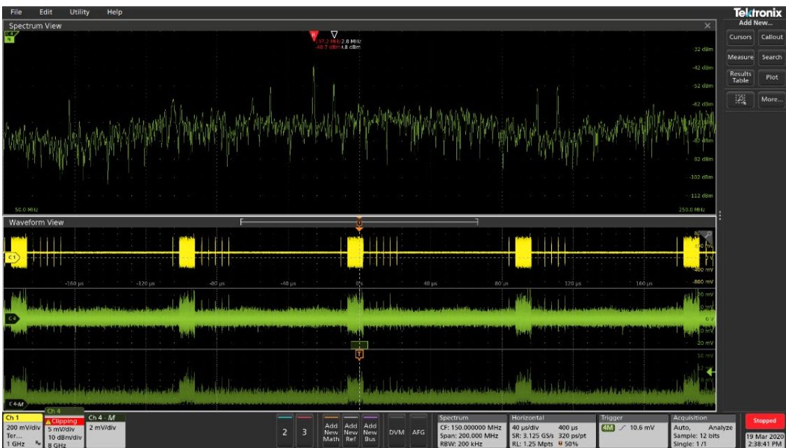
FIGURE 15. Trigger on RF Magnitude v Time on offending RF energy and observing the coincident electrical event.
